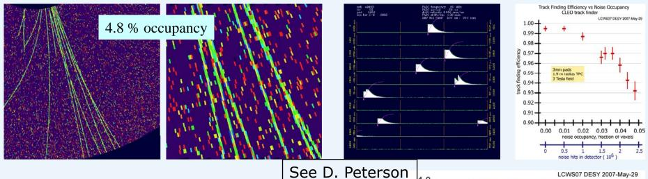
The effects of (salt and pepper) noise hits are studied by overlaying the FADC time response of track-related ionization with the response from the noise hits.
