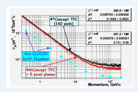
The Reduced scattering and point resolution are expected to provide improved momentum resolution.
