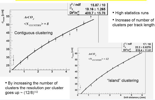
Two clustering methods were presented, with point resolution measurements.
