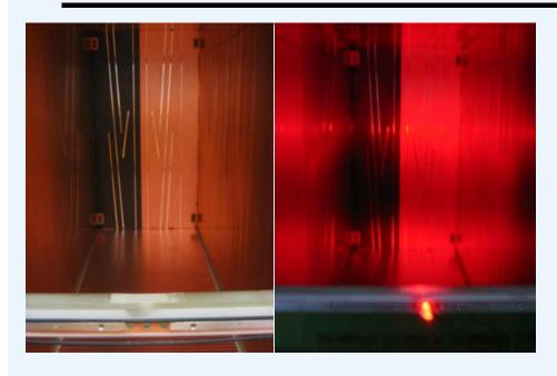
To produce photoelectrons for distortion measurements, place on the central cathode a pattern of metal with a lower work-function.
