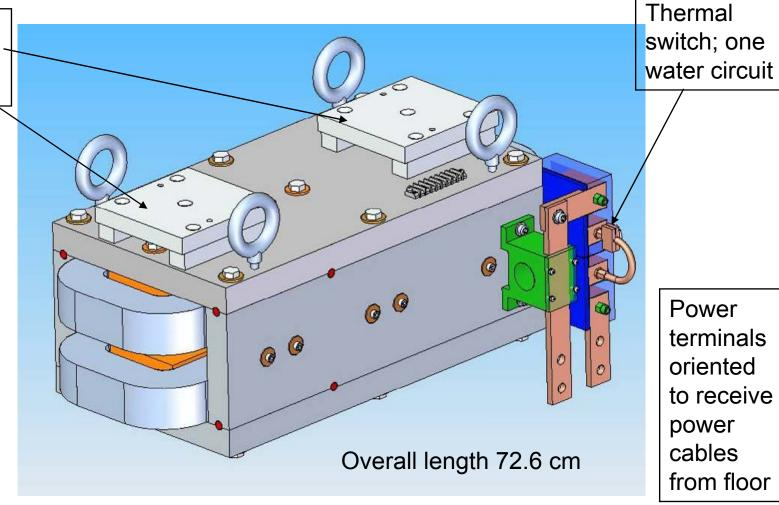
Power terminals oriented to receive power cables from floor
