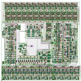
563 Transistors (2 buffers +calibration)
