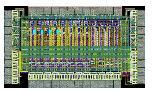
8 channels with continuous shaping and 4 channels with switched-reset
