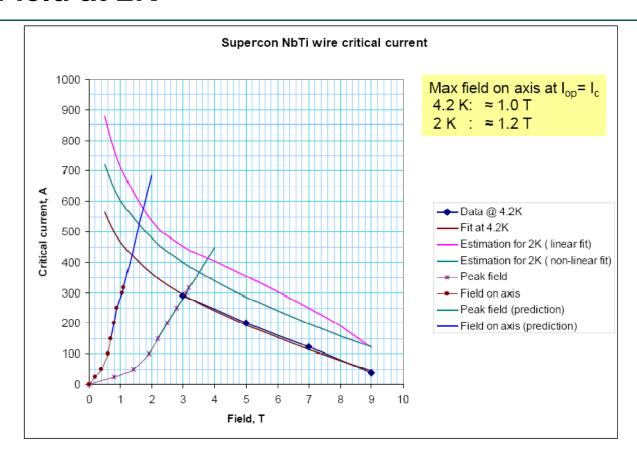
Lowering undulator working temp from 4 to 2K gives about 20% gain in the field on axis
