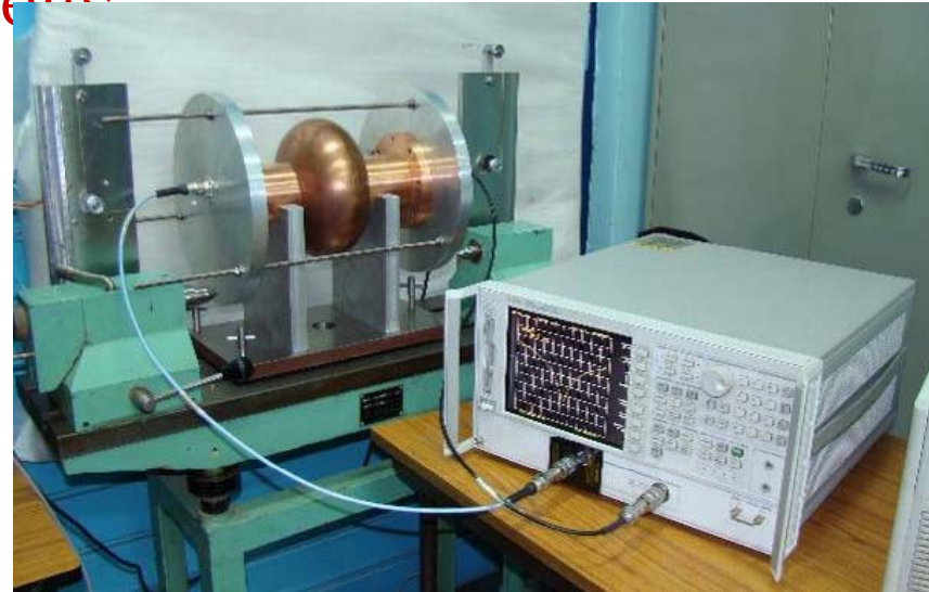
Bead Pull Measurement Setup for Assembled Cavity
