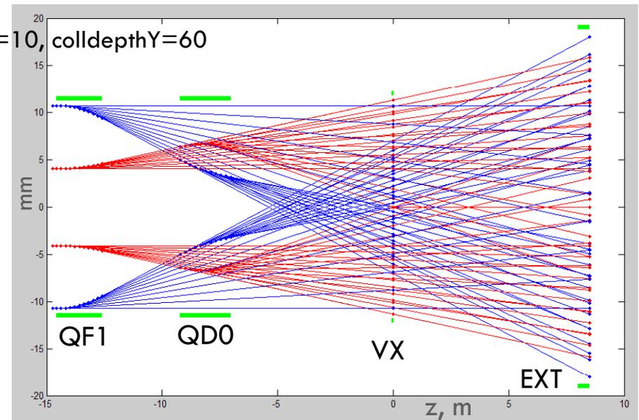
Rays show trajectories of possible SR photons. Amount of rays is not quantitative.
