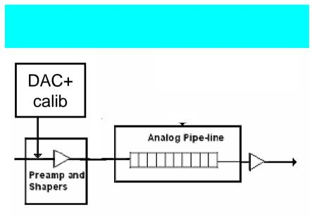
Last block to be tested (in progress). This the new pipeline developed by LAPP with an output buffer to isolate the pipeline output from parasitic capacitive effects.
