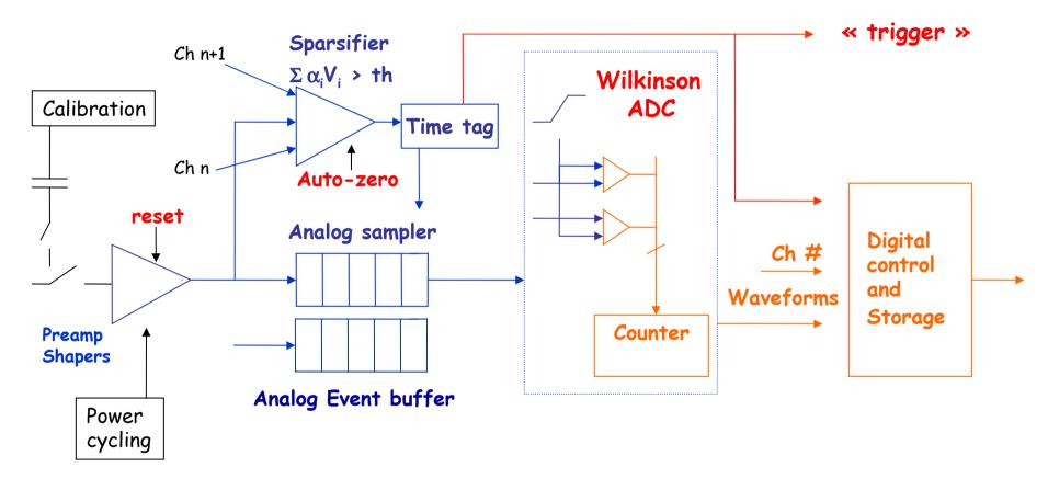
Charge 1-30 MIP, Time resolution: BC tagging 150-300ns 80ns analog pulse sampling
