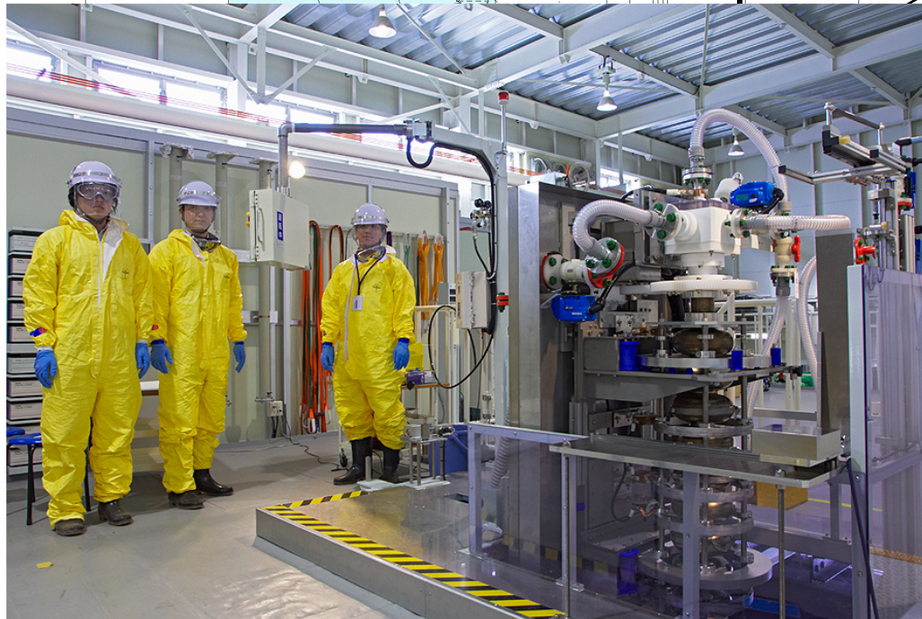
STF – EP system commissioning using old MHI cavity Picture shows acid draining by holding cavity up. 3 times EP cycle (40+60+60 \mu m removal) were done.
