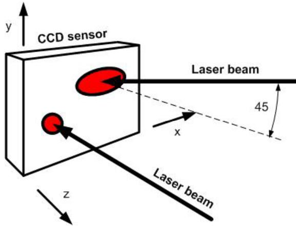
Two laser beams allow to measure displacements in xyz.
