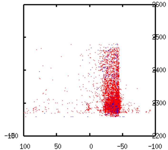
Particles (blue electrons/positrons, red photons) scattering back into the detector.
