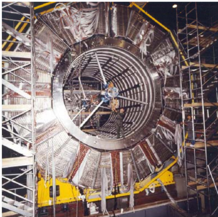
Hall probe measuring devices being set up in the coil
