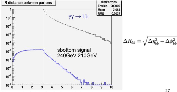
$\Delta R_{bb}$  separation for b-jets from background is always above  $\pi$  at the parton level
