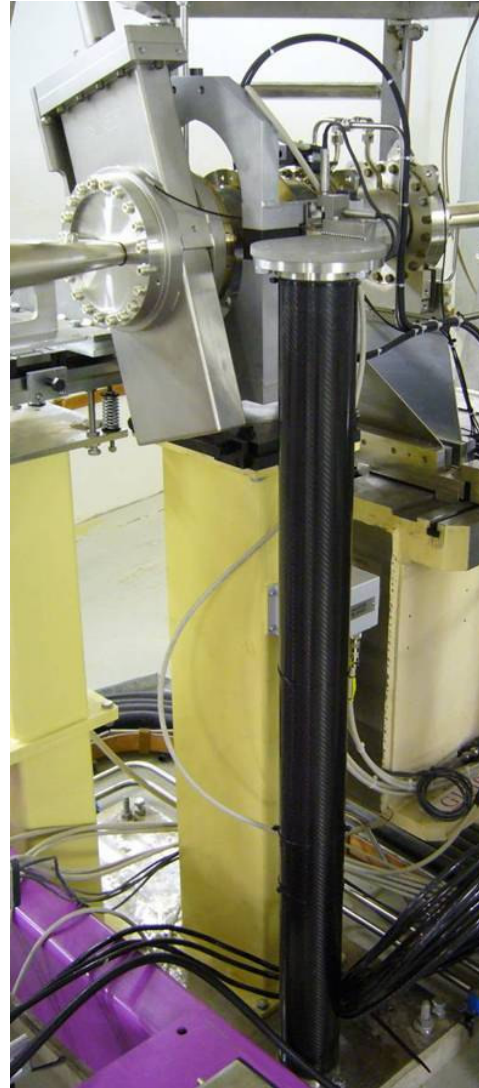
Reference pillar supporting linear encoders
