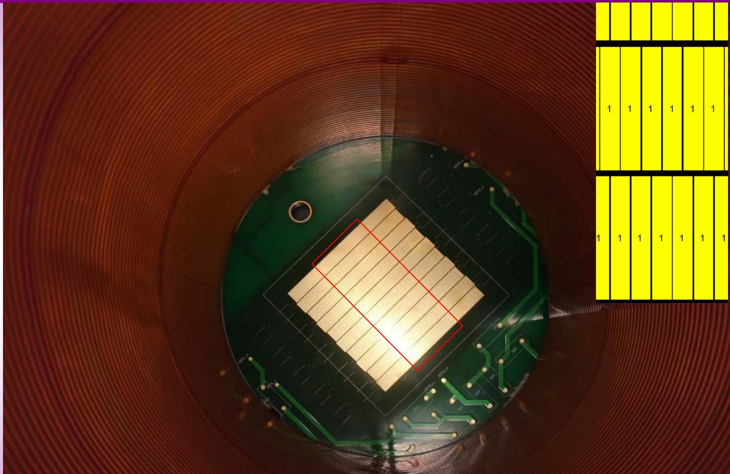
Readout pad: size,  $9.5\text{ mm} \times 1.5\text{ mm}$  (Pitch:  $10\text{ mm} \times 1.6\text{ mm}$ ), staggered
