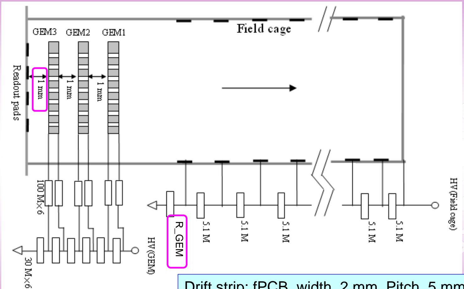
Drift strip: fPCB, width, 2 mm, Pitch, 5 mm
