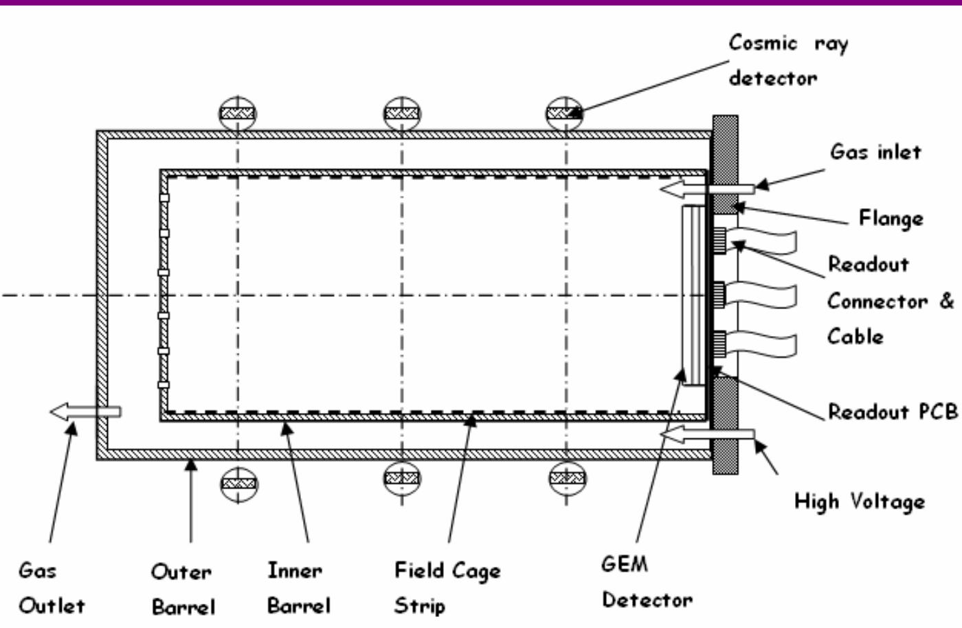
Readout detector: triple-GEM, CERN standard GEM foils, 10 cm × 10cm;
