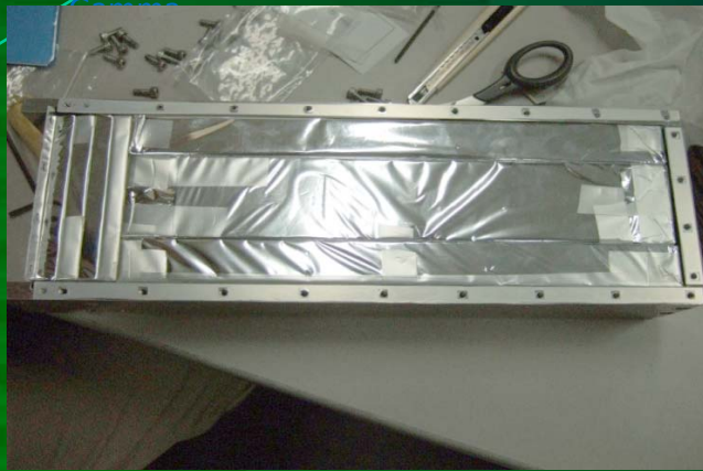
CsI(Tl) scintillator 4 front layers (5 mm thick each) + 1 bulk layer (290 mm thick)
