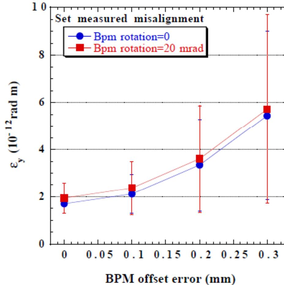
Magnet alignments ( $< 30\mu\text{m}$ ) are important,
