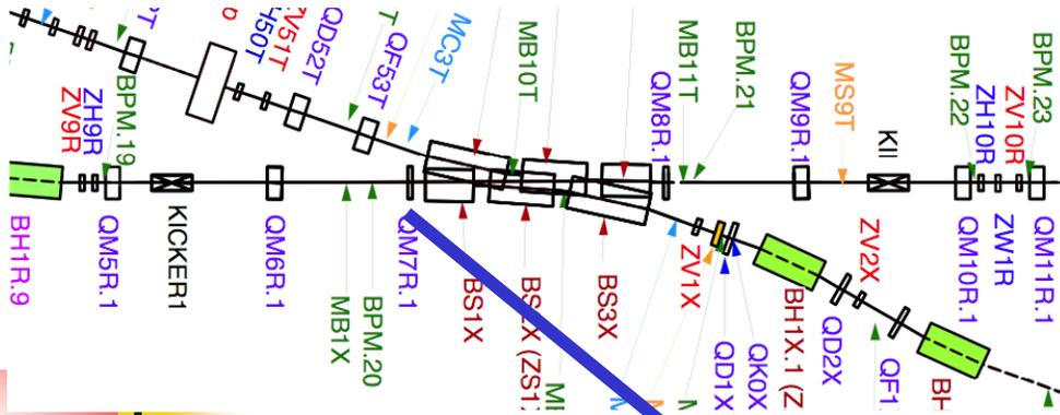
The aperture survey was carried out by using present magnets and DC power supplies. The required bump height is 5mm to separate the extraction beam and the circular beam.
