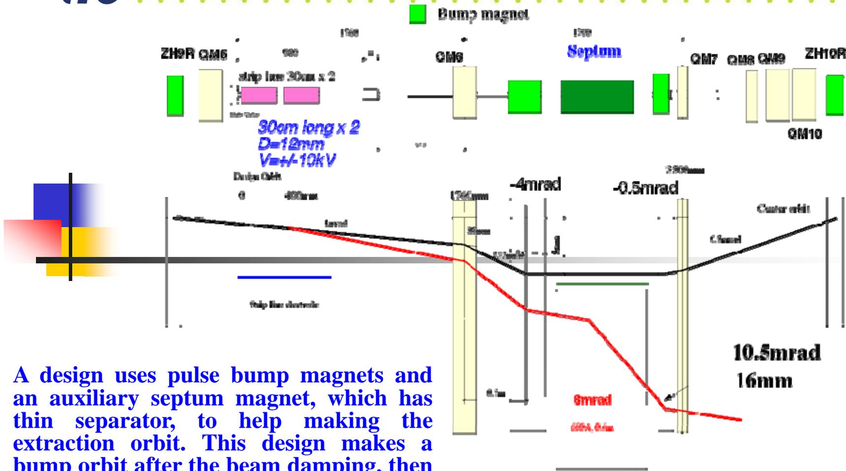
A design uses pulse bump magnets and an auxiliary septum magnet, to help making the extraction orbit. This design makes a bump orbit after the beam damping, then the selected bunch is extracted bunch-by-bunch by the strip-line kicker.
