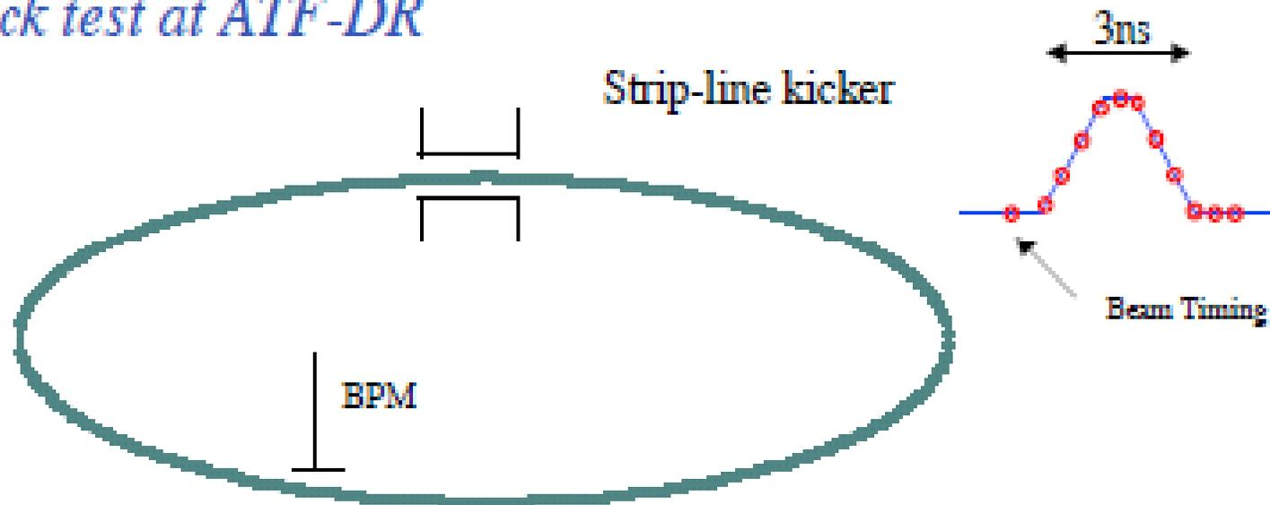
The kicker pulse is applied to the strip-line electrode at just the time of the beam goes through the electrode.
