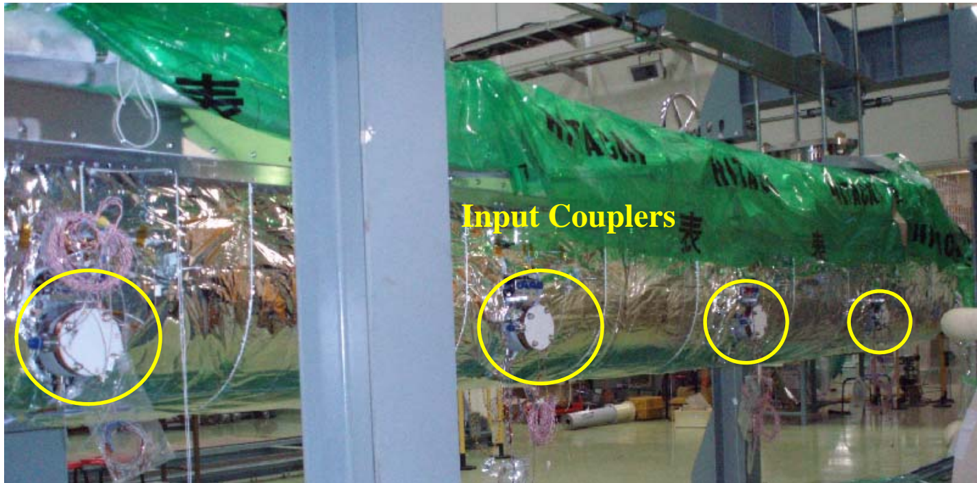
Super Insulations on the 5 K shield
