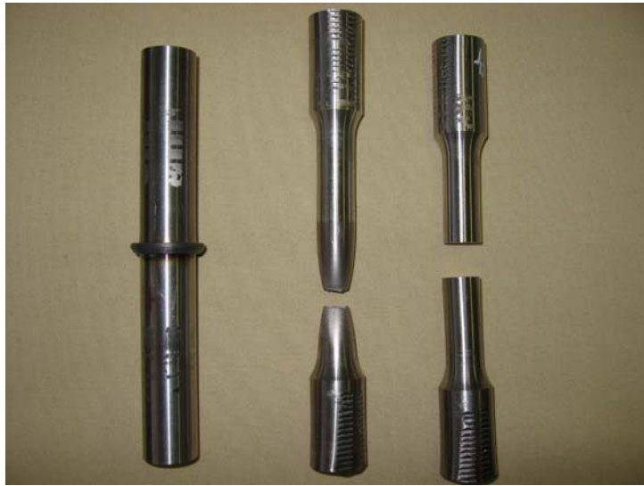
Sample of friction welded transition and broken samples after the tensile test
