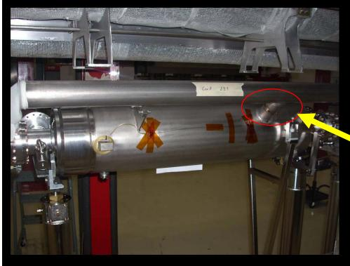
Allows making 2-phase line totally SS including all bellows
