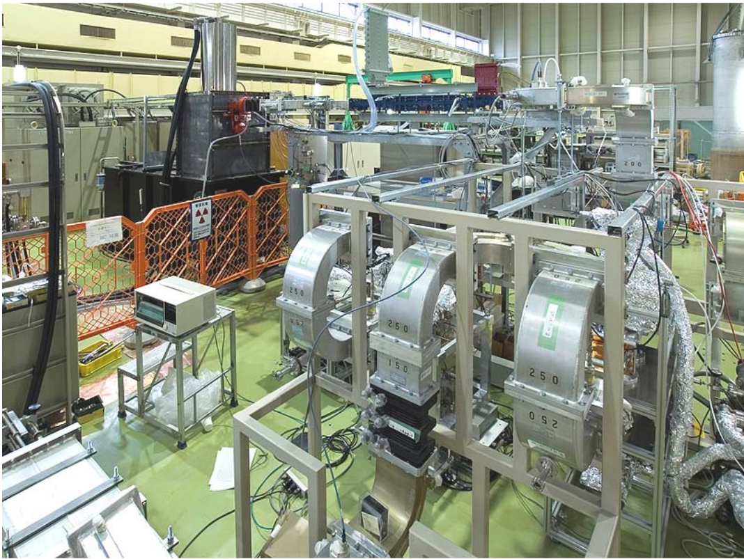
Waveguide to Distribute Power for Coupler Testing
