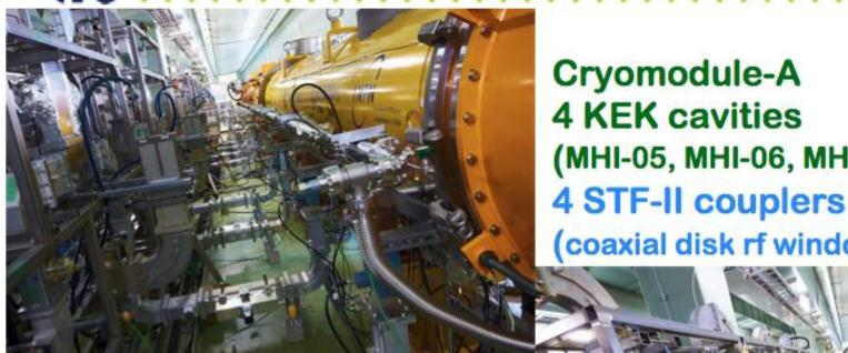
Cryomodule-A 4 KEK cavities (MHI-05, MHI-06, MHI-07, MHI-09)
