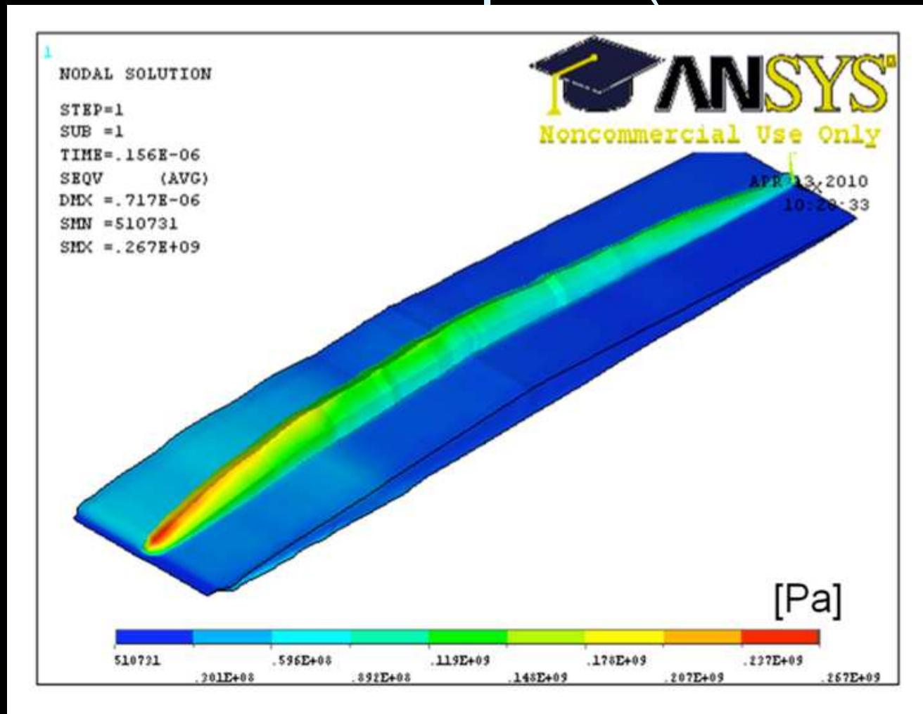
No risk of fracture, but collimators should be tested for compressive stresses up to 200 MPa.
