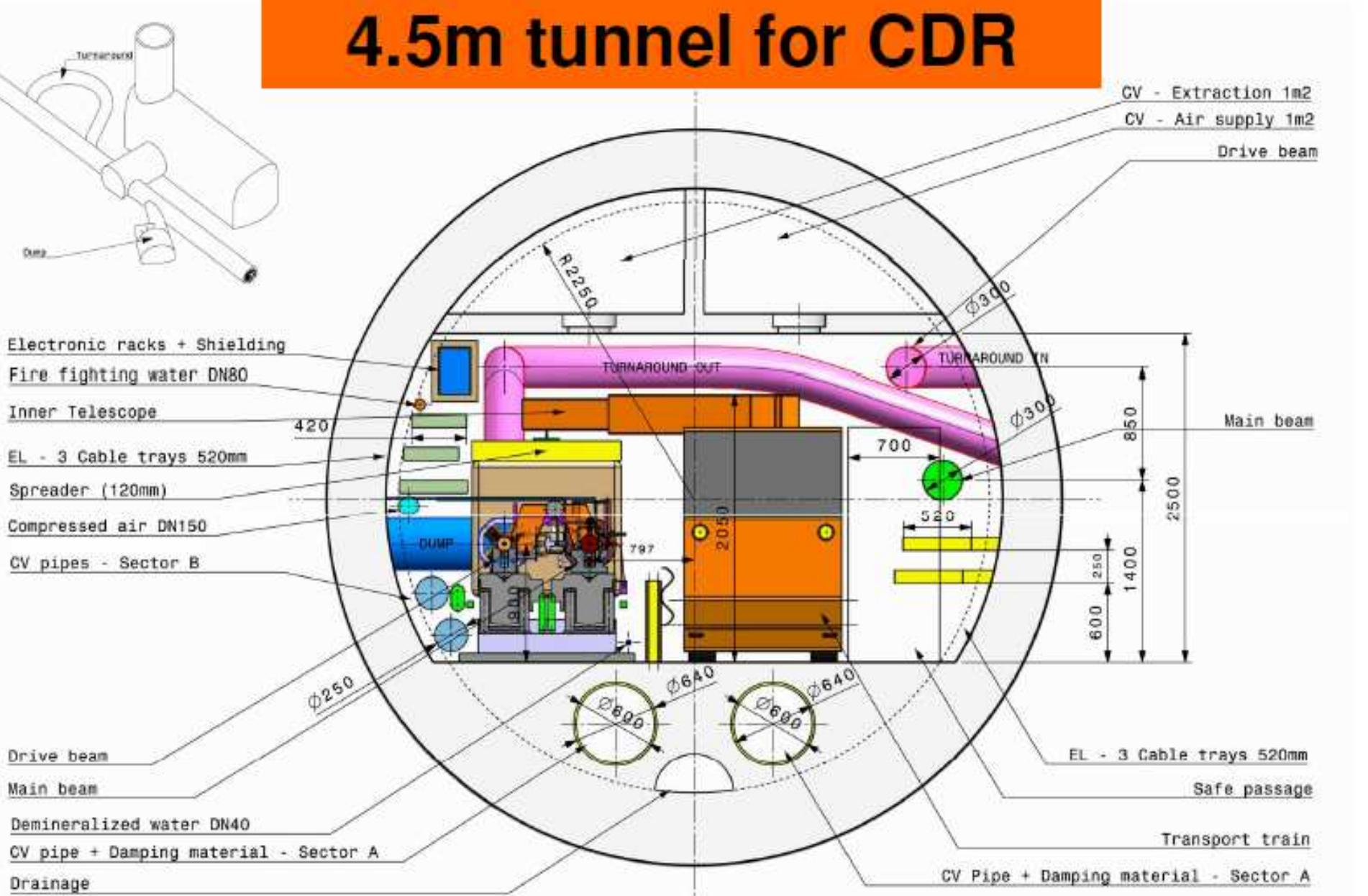
CLIC - Typical Cross Section - Diameter 4500mm - Junction with Turnaround - 1:25
