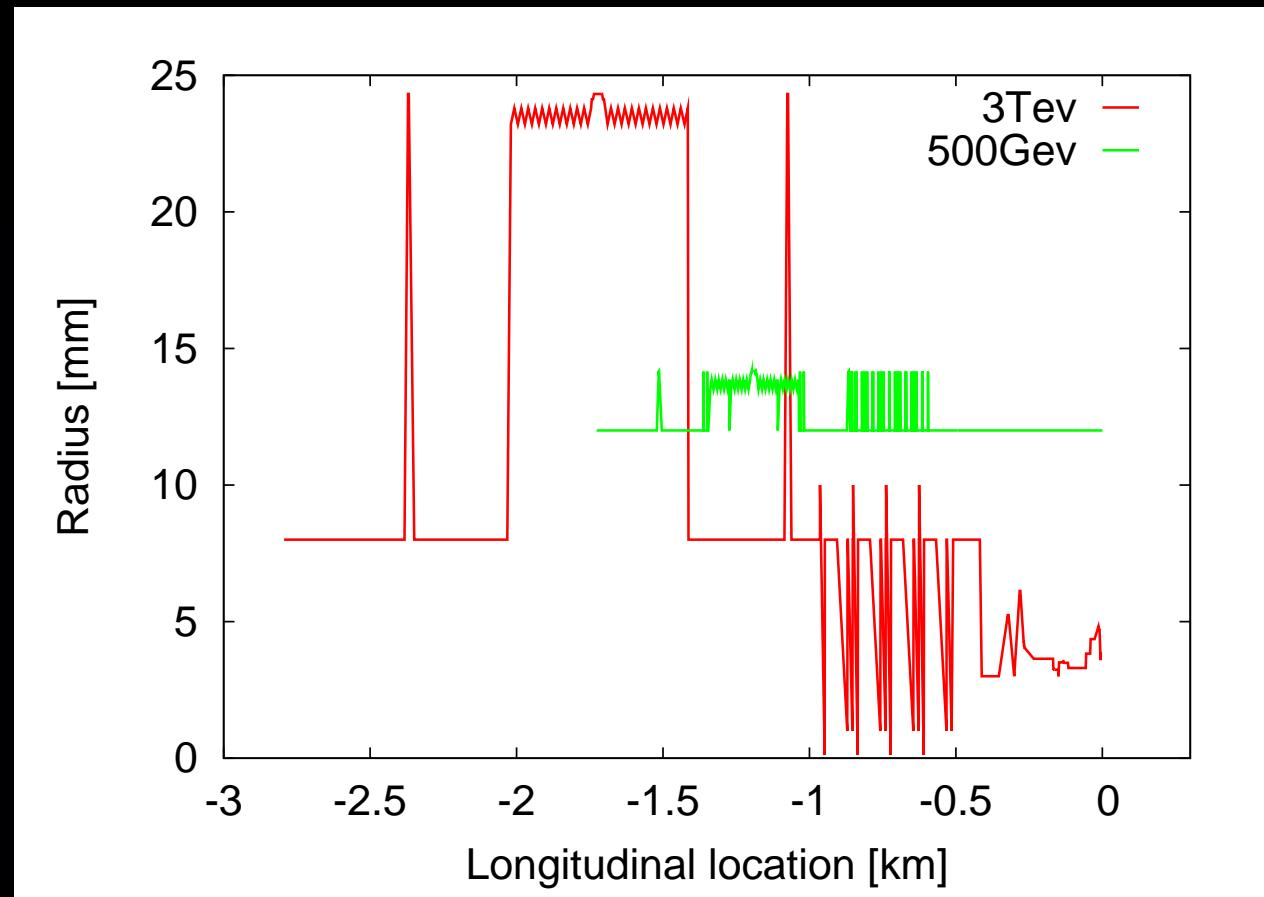
Reference beam pipe radius 8 mm at 3 TeV and 12 at 500 GeV. Tight apertures (3-5mm) at 3.5 TeV (FFS).
