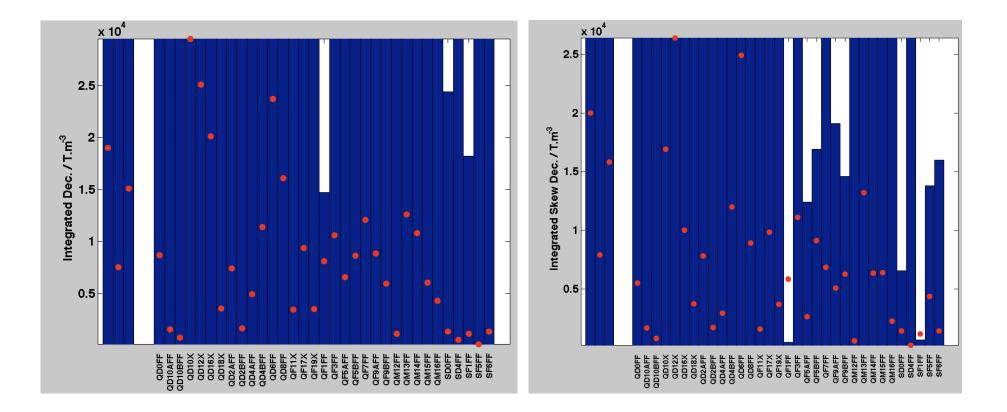
Dec & Skew-Dec multipole strength measurements and sensitivities
