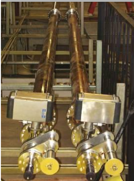
The ASTA pulse compressor with variable iris
