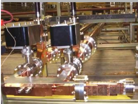
The ASTA pulse compressor with variable iris
