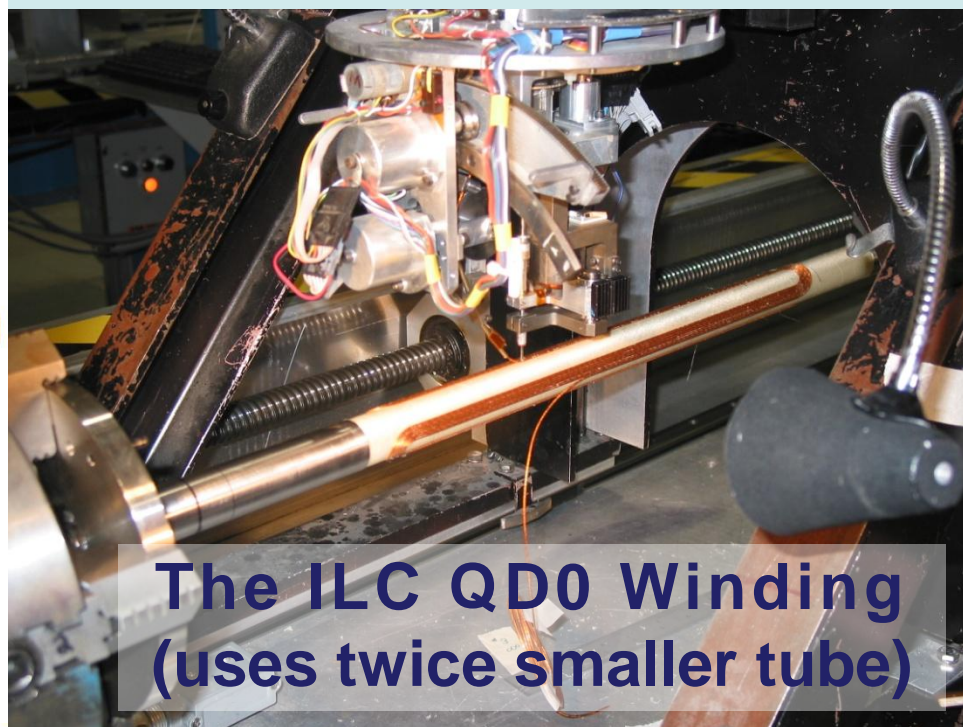
ILC QD0 Coil Pattern Concept (multi-layer, 7-strand cable winding)
