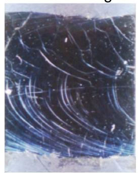
Thermal etching makes Grain boundaries visible
