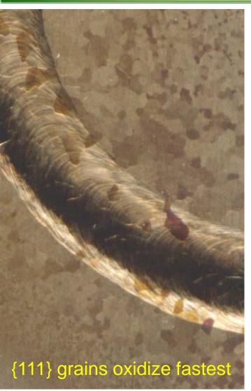
Differential oxidation after exposure to air before fully cooled delineates grains
