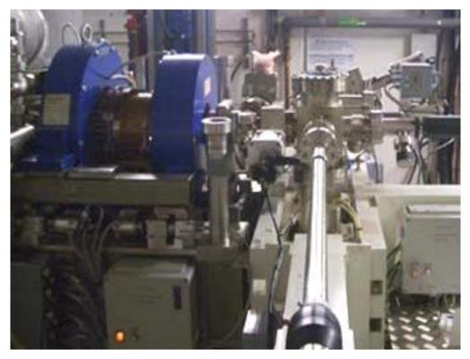
Photo injector area with rf gun cavity at FLASH
