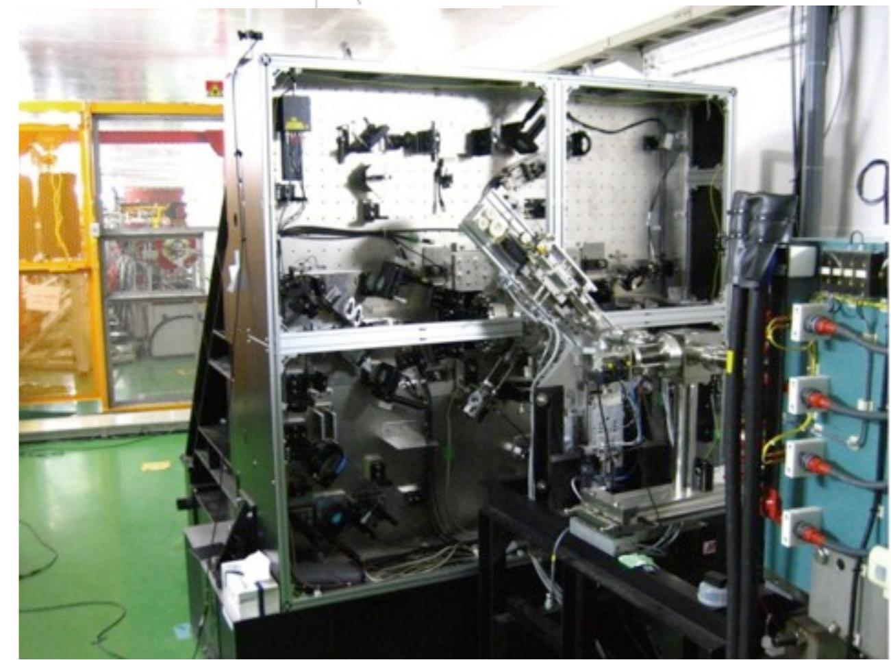
The vertical optical table installed at ATF2 beam line
