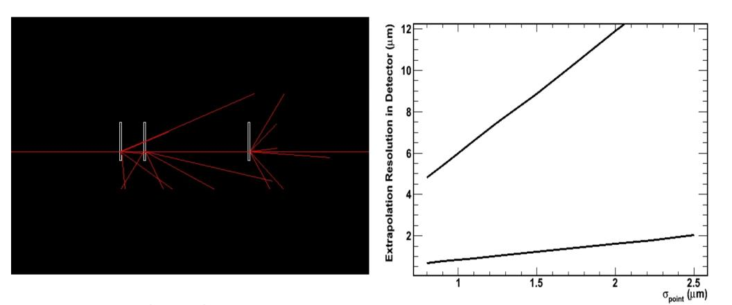
Generate lcio files of simulated SimTrackerHits and MCParticles to test reconstruction and extrapolation resolution;
