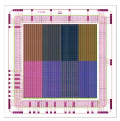
Test chip to optimise pixel cell for charge collection and back-gating effect mitigation;
