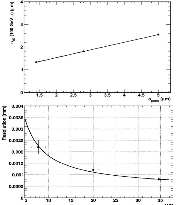
Scaling of asymptotic R-Φ impact parameter resolution (a) with single point resolution for a three double-layered barrel VXD in the CLIC geometry (100 GeV single muons with Mokka+MarlinReco);
