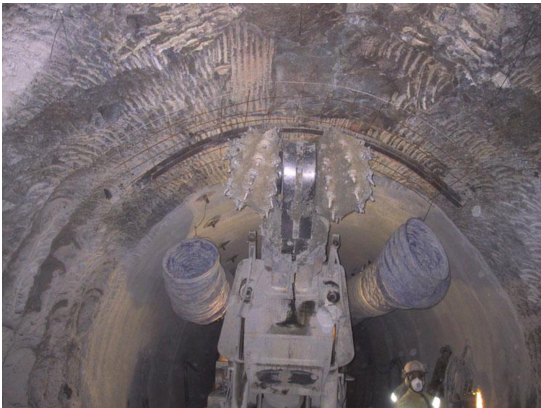
Fig. 6.2.5-1: Roadheader type machine
