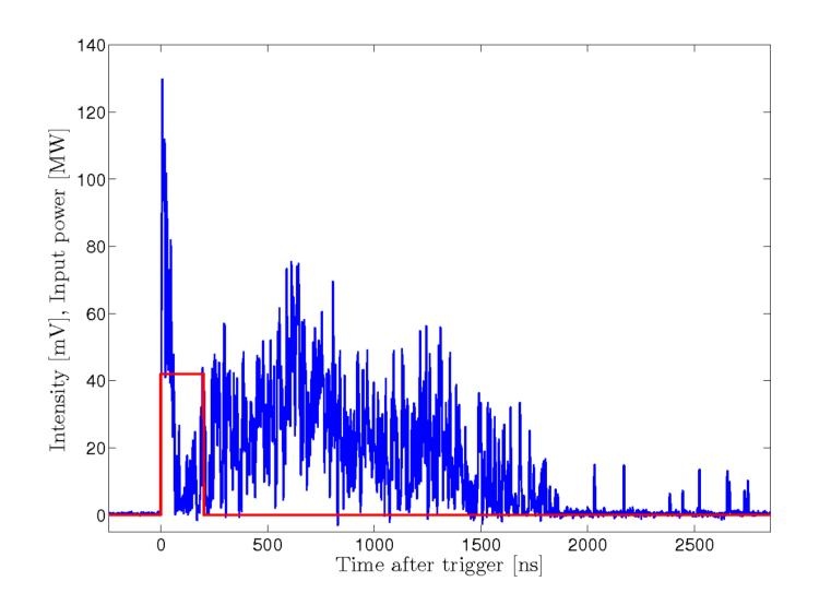
Total emitted light intensity (blue) and rf input power (red) of an rf breakdown, the first sharp peak can be attributed to strong OTR.
