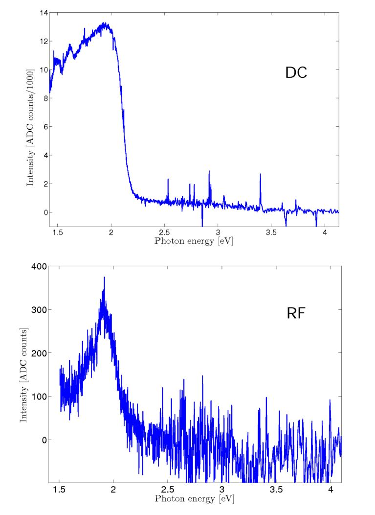
Breakdown spectrum in dc and rf on Cu. Removal of CuO layer (~ 150nm) due to conditioning.
