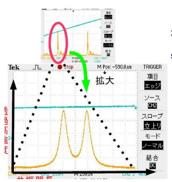
3D 4M cavity resonates with left and right circular polarization separately
