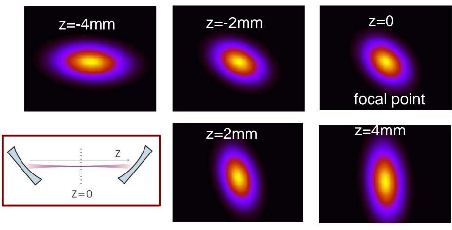
profile is rotating during its propagation! angular momentum of light
