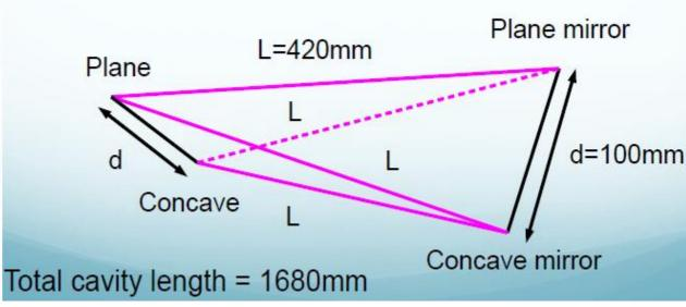
optical feature of the 3D4M cavity is being studied on test bed
