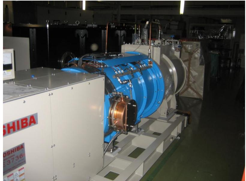
In FY2009 at KEK, a 10MW horizontal klystron is procured but due to the poor resource, it has not yet operated.
