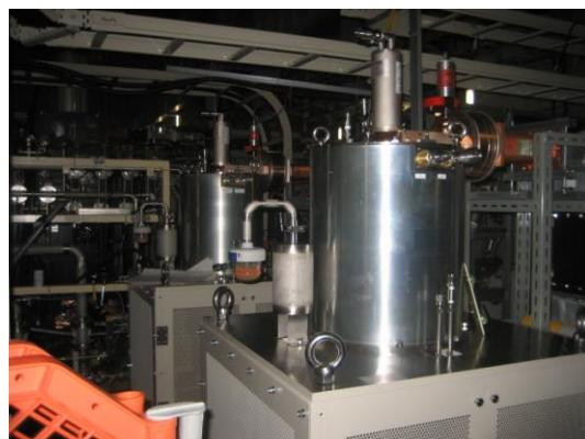
Two prototype DRFS klystrons
