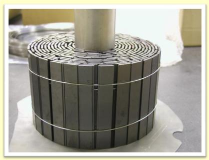
SiC prepared for baking at 950 deg C
