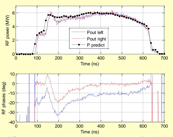
PETS is a very sensitive diagnostics for the longitudinal beam structure, IQ-detectors used for power measurements
