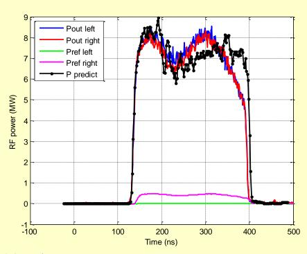
20 MW power produced with a 10A beam according to predictions, form factor 0.9
