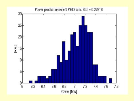
Current stability  $\sim 1.3\%$ ; P  $\sim I^2$ Measured current stability in the CTF3 linac  $9\times10^{-4}$
