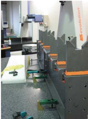
SiC girder before final Grinding at Boostec
