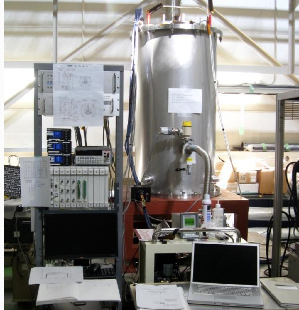
KEK Test Stand to test the quadrupole in the conduction cooling mode
