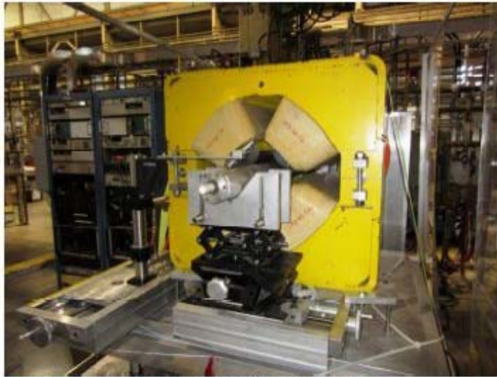
Figure 1: 4Q17 magnet with rotating coil and feedthrough holder setup
