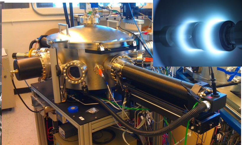
High-impulse deposition at LBNL
