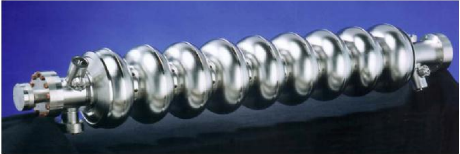
Figure 1.2-1: A TESLA nine-cell 1.3 GHz superconducting niobium cavity.
