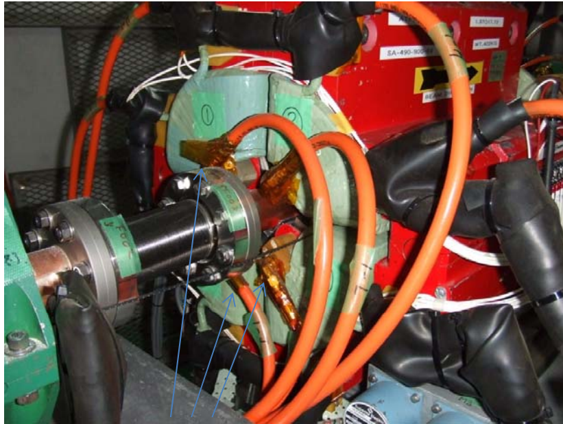
Connector of cooling water (Iron) Connector of magnet is stainless steel
