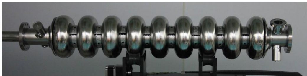
PKU No.04(Large Grain; TESLA Shape) 2nd. Vertical Test 04/25/2013 Local Grinding, EP-II(20 \mu\text{m} ), Water flow(1.5hrs), FM_20 2%(50C,60min), H.P.R.(~7hrs), Baking(140C, 44hrs)
