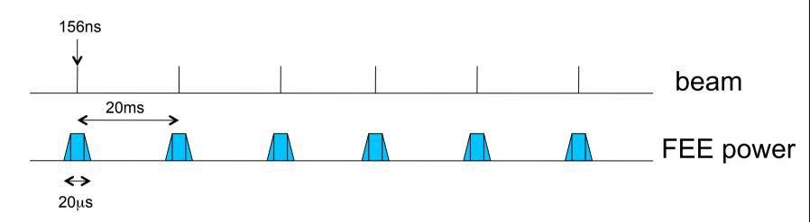
The analog part of the FEE is powered for only 20  $\mu$ s every 20ms and the average power over one second is reduced to a small fraction of the peak power. Similar scheme applies to all the sub-detectors, with the only possible exception of the muon chambers.
