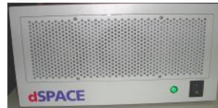
dSPACE Real time hardware for Rapid Control Prototyping
