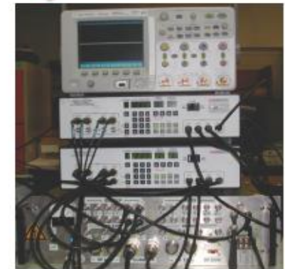
Amplifiers, filters input/output board for signal conditioning
