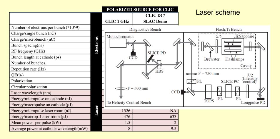
For the 1 GHz approach cathode current densities of 3-6 A/cm<sup>2</sup> would be needed, the dc approach uses < 1 A/cm<sup>2</sup>
