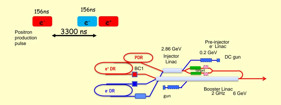
Save two rings, positron driver linac, and tunnel length (saving potential 200 MCHF)
