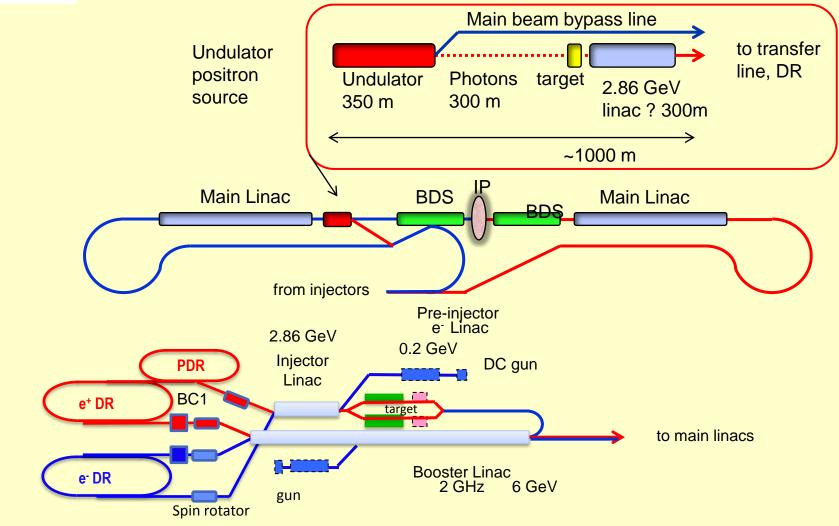
Minimum scenario for upgrade to positron polarization and fully compatible with conventional layout
