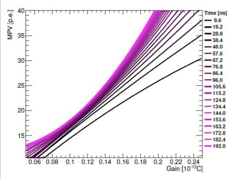
For short integration times ( < recovery time of MPPC micro-cells): Linear dependence of MIP on gain
