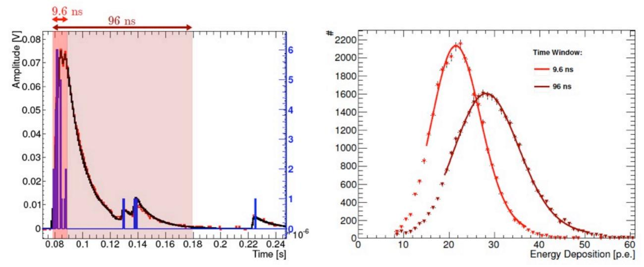
MIP amplitude in p.e. depends strongly on integration time: Afterpulses of the photon sensor!
