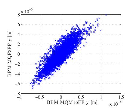
Measured vertical beam position data of the BPMs 111 (left) and 112 (right) versus BPM 134. A strong change in correlation can be seen.
