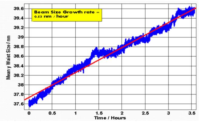
Reminder- when get close to goal, beam size drift as function of time due to measured ground motion should become noticeable
