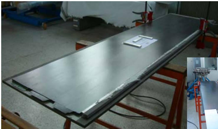
The 1 st long layer of 3 alveoli demolded (186,8 x 6,5 mm x 2,5m – 0,5 mm thick)
