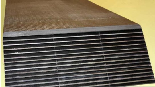
From the structure of a real module (barrel or End-cap) Thick plate / alveoli / tungsten...
