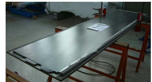
The 1 st long layer of 3 alveoli demolded (186,8 x 6,5 mm x 2,5m – 0,5 mm thick)
