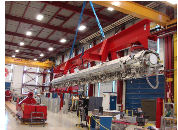
Movement of cold mass to Big Bertha cantilever fixture
